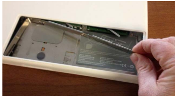
Figure 3 - Remove L-shape cover
