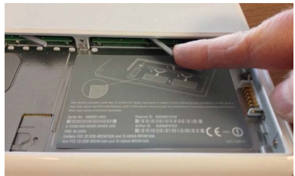
Figure 4 - Push metal lever to remove RAM
