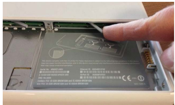
Figure 4 - Push metal lever to remove RAM
