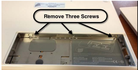
Figure 2 - Remove three screws
