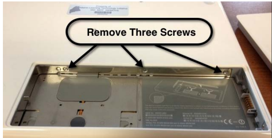
Figure 2 - Remove three screws
