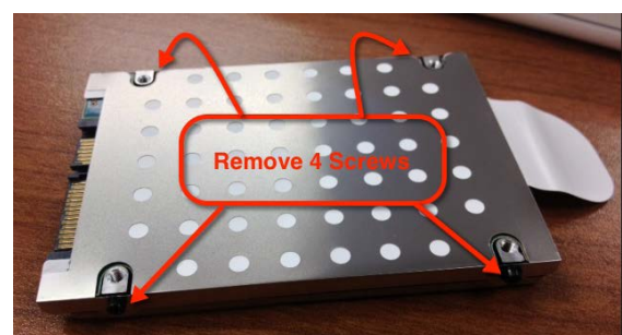
Figure 5 - Remove four T-8 Screws
