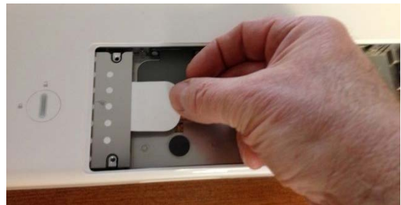
Figure 4 - Pull the plastic tab to remove HD
