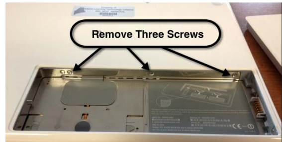
Figure 2 - Remove three screws
