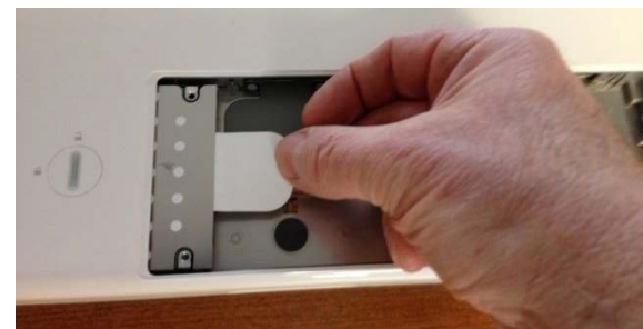
Figure 4 - Pull the plastic tab to remove HD
