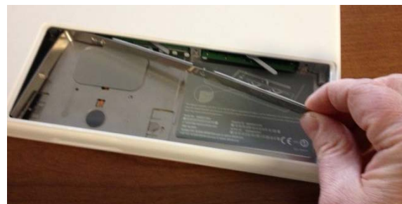
Figure 3 - Remove L-shape cover
