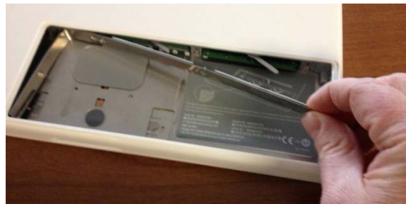
Figure 3 - Remove L-shape cover
